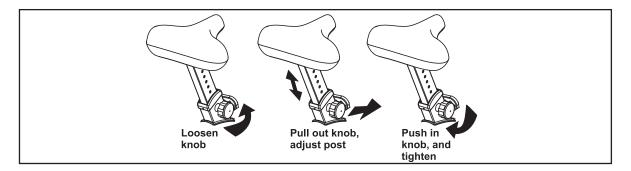
**CAUTION :** When using the height adjustment mechanism to change the height of a partially raised seat, hold the seat to prevent it from falling on the hand.
